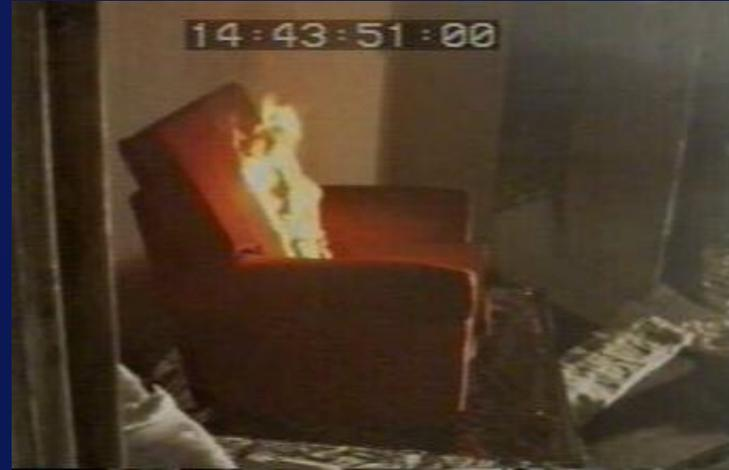
An experiment involving fire in a modern armchair. The room is connected through an open door to other rooms of the house.
