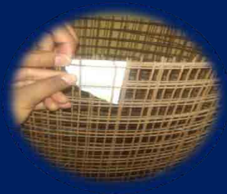
Welded wire Mesh (WWM)
