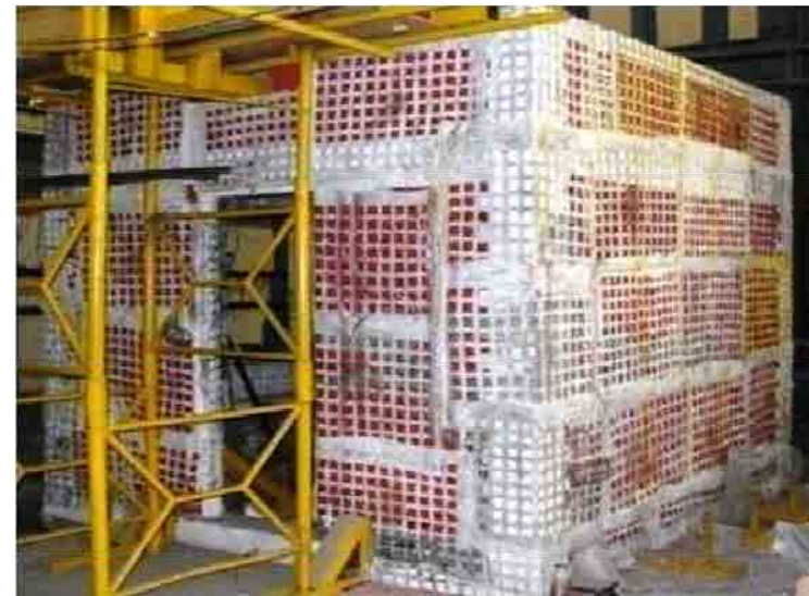
Application of Plastic Cement Bag Mesh
