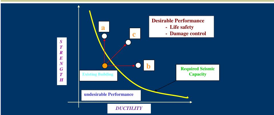
a. to increase the ultimate strength of overall structure, *RC wall, Steel Framed Brace*
