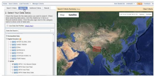
5. Next click on Datasets Tab on top→of the datasets opened on left panel move to Digital Elevation→Click on SRTM→Select SRTM 1 Arc Second Global data→Click on Search Tab at bottom.
